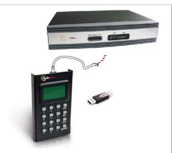
For PED-authenticated Luna G5, connect the PED at the front panel, using the provided local PED cable – applies only for PED-authenticated HSM; otherwise skip to the next step.
